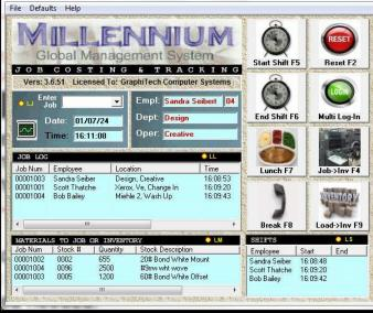
Each Data Collection Terminal (as shown to the left), can be set up in each department and programmed to reflect the activity of that department (minimizes data entry).
