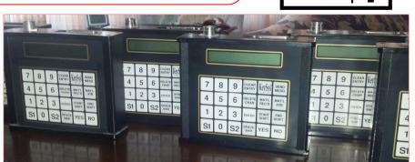
membrane cover and contains provisions for sending messages, receiving messages, using hot keys, bar code input, entering of materials, and maintaining real-time verification of entered data. KeySys keypads may be installed flat on a desk or attached to a wall or post using our acrylic and/or steel mounting brackets. A 2-line display of 24 characters each provides feedback for all data entry.
